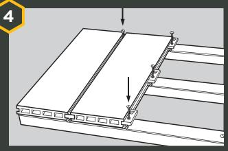
Take the next piece of deck and securely push into the Universal Clips. Now nip the screw to secure the Universal Clip against the board. Do not over tighten. Now repeat steps 3 and 4 to cover the deck, using one Universal Clip and screw on every joist.
