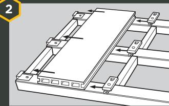
Place the first piece of decking on the timber frame with the decking running perpendicular to the joists. The first piece of deck may be secured with starter clips. **Do not** screw or nail through HD Deck® 150, use one Universal Clip and screw on every joist.
