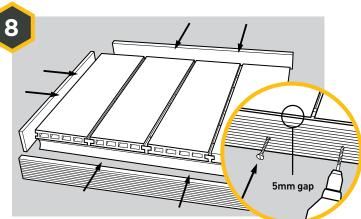
If using fascia, drill pilot holes with counterbore through the fascia at 200-300mm intervals. According to ambient temperature allow a **5-7mm gap** between end of deck board and the fascia. Screw fascia to the joist. Always screw fascia to the joist at a 90° degree angle.
