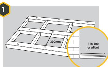
We recommend using treated 47x100mm timber joists and building in a gradual gradient of at least **1 in 100** (1%) that runs away from any adjoining buildings. Boards should run lengthways down this gradient to help water naturally disperse.
