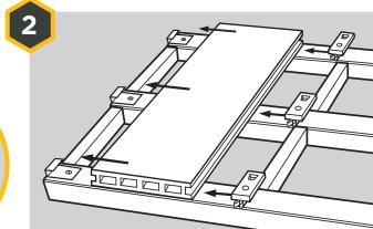
Place the first piece of decking on the timber frame with the decking running perpendicular to the joists. The first piece of deck may be secured with starter clips. **Do not screw or nail through** *HD Deck®* **150**, use one Universal Clip and screw on every joist.
