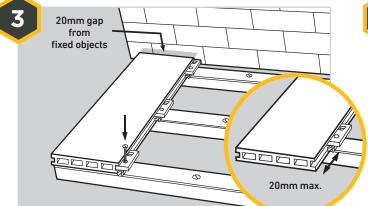
To secure the first board, use one Universal Clip and screw on every joist. Take a screw, place in the hole located in the Universal Clip and screw into the wooden joist. **Do not tighten at this stage**. Make sure the boards do not overhang the joist at the edge by **more than 20mm** and a **20mm expansion gap** should be left between the wall or other fixed objects surrounding the deck.
