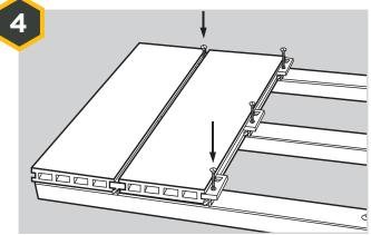
Take the next piece of deck and securely push into the Universal Clips. Now nip the screw to secure the Universal Clip against the board. **Do not over tighten**. Now repeat steps 3 and 4 to cover the deck, using one Universal Clip and screw on every joist.
