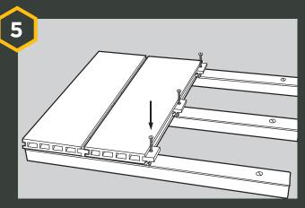
Now repeat steps 3 and 4 to cover the deck, using 1 clip and screw on every joist.
