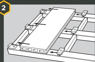
Place the first piece of decking on the timber frame with the decking running perpendicular to the joists. The first piece of deck may be secured with starter clips. **Do not screw or nail through** *HD Deck® 150*, use 1 clip and screw on every joist.
