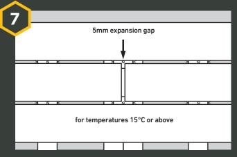
**IMPORTANT:** Do not allow deck boards to meet at the ends. When installing in temperatures of:
