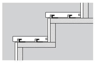
Install the HD Deck® Dual bullnose deck board as per the above instructions, leaving a gap behind the board to enable you to fit the fascia.
