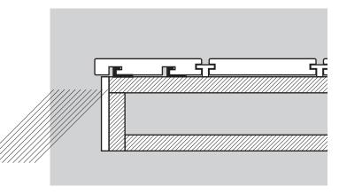
After installing the *HD Deck® Dual* bullnose deck board, as per the above instructions, use the Universal Clip to secure to the rest of the deck. See *Using the New Universal Clip* overleaf.
