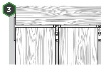
Repeat this process for the remaining deck boards, making sure the fronts of all the Universal Clips are firmly in the groove of the bullnose deck board.
