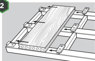
Place the first piece of decking on the timber frame with the decking running perpendicular to the joists. The first piece of deck may be secured with starter clips. **Do not screw or nail through** *HD Deck® Dual*, use one Universal Clip and screw on every joist.
