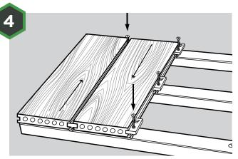
Take the next piece of deck and securely push into the Universal Clips. Now nip the screw to secure the Universal Clip against the board. **Do not over tighten**. Now repeat steps 3 and 4 to cover the deck, using one Universal Clip and screw on every joist. For a more natural finish, we recommend **alternating the direction of the wood grain** when installing the boards. If using the bullnose board, use this as your starting point.
