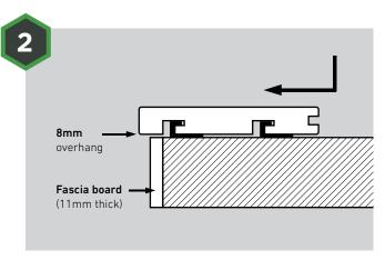
Insert the *HD Deck® Dual* bullnose deck board over the clips and push it forward. Secure in place with Universal Clips as required.
