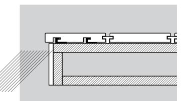
After installing the *HD Deck® Dual* bullnose deck board, as per the above instructions, use the Universal Clip to secure to the rest of the deck. See **Using the New Universal Clip** overleaf.
