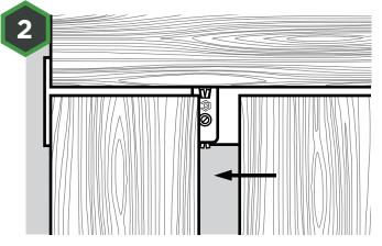
Screw the Universal Clip to the joist, then securely push the next deck board in place.
