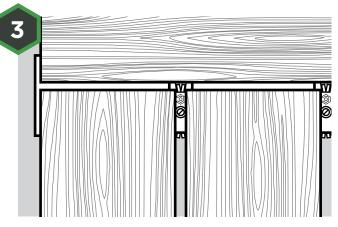
Repeat this process for the remaining deck boards, making sure the fronts of all the Universal Clips are firmly in the groove of the bullnose deck board.
