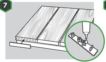
If using end caps, apply a high quality grab adhesive to the end caps to secure for extra adhesion. Wipe away any excess from the edge of the cap.
