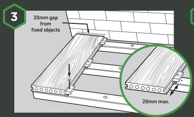
Take a screw, place in the hole located in the clip and screw into the wooden joist. Do not tighten at this stage. Make sure the boards **do not** over hang the joist at the edge by more than 20mm and a 20mm expansion gap should be left between the wall or other fixed objects surrounding the deck.
