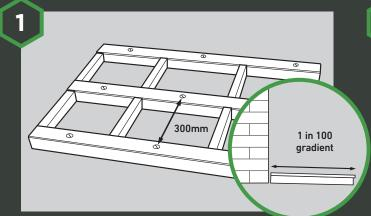
We recommend using treated 47x100mm timber joists and building in a gradual gradient of at least 1 in 100 (1%) that runs away from any adjoining buildings. Boards should run lengthways down this gradient to help water naturally disperse.
