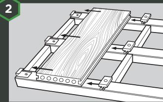
Place the first piece of decking on the timber frame with the decking running perpendicular to the joists. The first piece of deck may be secured with starter clips. **Do not** screw or nail through HD Deck® Dual, use 1 clip and screw on every joist.
