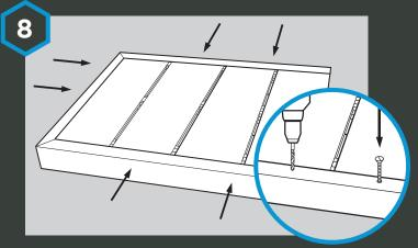
If using, take the angle edging strip and place on the edge of the deck. Allow a **5mm gap** between end of deck board and vertical edge of the strip. Use a drill to first make a pilot hole through the strip and deck. Screw strip into the joist through the first pilot hole. Drill more pilot holes as required and affix strip with screws.
