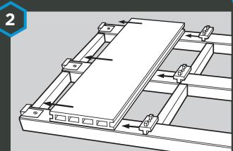
Place the first piece of decking on the timber frame with the decking running perpendicular to the joists. The first piece of deck may be secured with starter clips. **Do not screw or nail through** *HD Deck® XS*, use 1 clip and screw on every joist.
