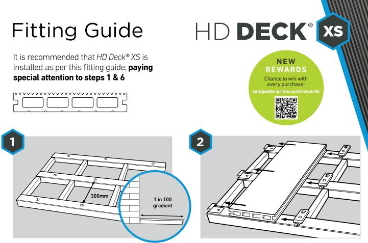
We recommend using treated 47x100mm timber joists and building in a gradual gradient of at least **1 in 100** (1%) that runs away from any adjoining buildings. Boards should run lengthways down this gradient to help water naturally disperse.
