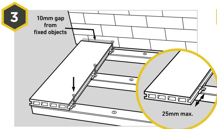
To secure the first board, use one Slim Clip and screw on every joist. Take a screw, place in the hole located in the Slim Clip and screw into the subframe. Make sure the boards do not overhang the joist at the edge by **more than 25mm** and a **10mm expansion gap** should be left between the wall or other fixed objects surrounding the deck.
