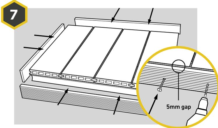
If using Fire Fascia, drill pilot holes with counterbore through the fascia at 200-300mm intervals. According to ambient temperature allow a **5-7mm gap** between end of deck board and the fascia. Screw fascia to the joist. Always screw fascia to the joist at a 90° degree angle.
