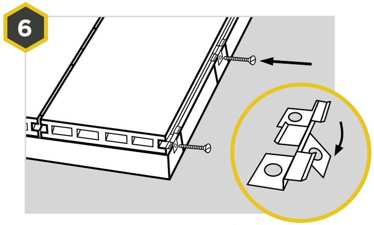
In order to fit the final board, bend the Slim Clip screw hole to a **90° angle** and fit over the edge of the subframe. Screw into place to secure boards. If necessary, you can trim the excess tabs off.
