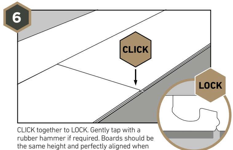
CLICK together to LOCK. Gently tap with a rubber hammer if required. Boards should be the same height and perfectly aligned when locked properly. If you are not using existing beading boards, expansion gaps can be finished with matching Touchstone trim that can be attached to the walls.
