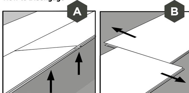
**A** Lift entire row of boards to 20° angle, disengage from main floor.
