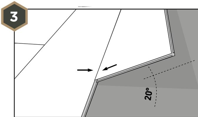
Beginning the next row, use remainder of cut plank from last piece of first row, provided piece is minimum 300mm. Otherwise cut a new plank to begin this row, ensuring joints are at least 180mm apart. Use the remainder of cut planks for ends of rows to begin subsequent rows whenever possible.
