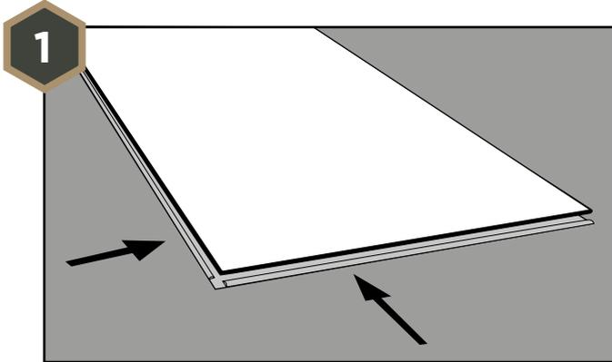
Once sub-floor is fully cleaned and prepared, begin with laying planks left to right for first row. Place first plank so grooved edge is facing towards you.
