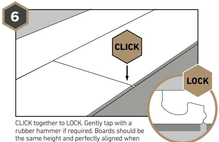
CLICK together to LOCK. Gently tap with a rubber hammer if required. Boards should be the same height and perfectly aligned when locked properly. If you are not using existing beading boards, expansion gaps can be finished with matching Touchstone beading that can be attached to the walls.
