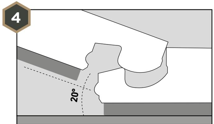
Click together the long sides of the new plank and the one in the previous row, placing the board tightly to the short end of the previous plank in this row with an angle of 20°. Drop the plank, and push to lock firmly together. These should be the same height if laid properly. Ensure both are perfectly aligned.
