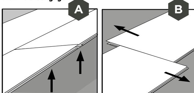
**A** Lift entire row of boards to 20° angle, disengage from main floor.
