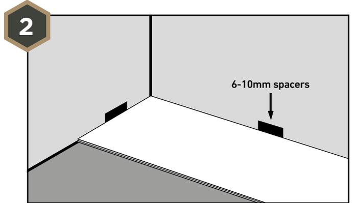
Insert 6mm spacers (minimum) between the wall and plank. Please consider that the expansion rate is 0.1% average. Lay the next board in the row interlocking with the first end-to-end and click to lock together. These should be the same height. Ensure alignment, then continue in same method.
