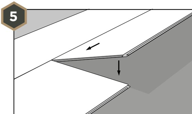
Slide board into position and drop into place.
