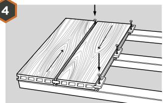
Take the next piece of deck and securely push into the Universal Clips. Now nip the screw to secure the Universal Clip against the board. **Do not over tighten**. Repeat steps 3 and 4 to cover the deck, using one Universal Clip and screw on every joist.
