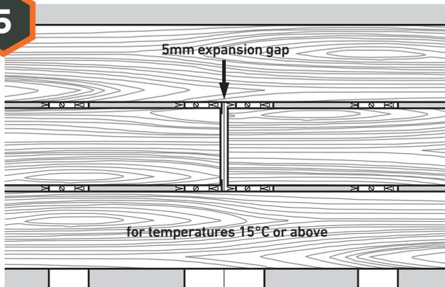
**IMPORTANT:** Do not allow deck boards to meet at the ends. When installing in temperatures of:
