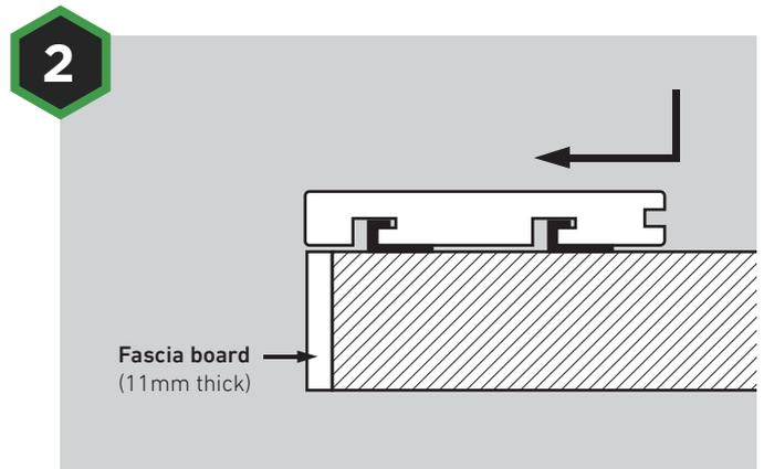
Insert the *HD Deck Dual*® bullnose deck board over the clips and push it forward. Secure in place with Universal Clips as required.
