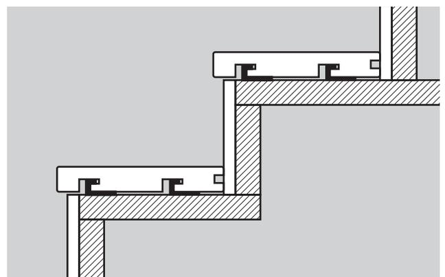
Install the *HD Deck Dual*® bullnose deck board as per the above instructions, leaving a gap behind the board to enable you to fit the fascia.
