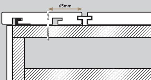
After installing the *HD Deck Dual*® bullnose deck board, as per the above instructions, use the Universal Clip to secure to the rest of the deck. See **Using the New Universal Clip** overleaf.
