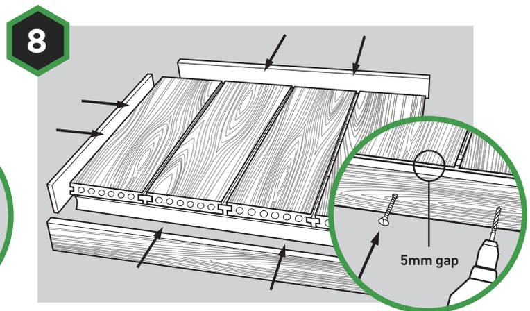
If using fascia, drill pilot holes with counterbore the fascia at 200-300mm intervals. According to ambient temperature allow a **5-7mm gap** between end of deck board and the fascia. Screw fascia to the joist. Always screw fascia to the joist at a 90° degree angle.
