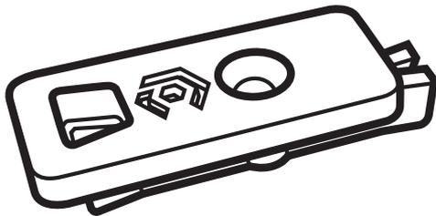
**Overhanging front end** for bullnose deck board installation
