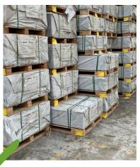
Max stack - 6 pallets high HD Deck should be stacked no higher than 6 on original pallets.
