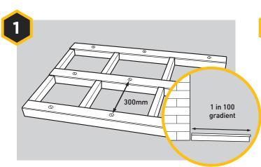
We recommend using a similarly fire rated subframe and allow for a gradual gradient of at least **1 in 100** (1%) that runs away from any adjoining buildings. Boards should run lengthways down this gradient to help water naturally disperse.
