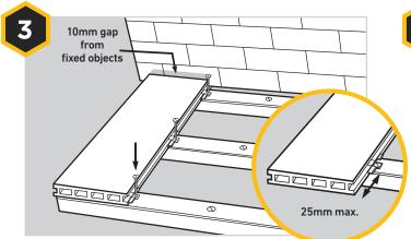
To secure the first board, use one Slim Clip and screw on every joist. Take a screw, place in the hole located in the Slim Clip and screw into the subframe. Make sure the boards do not overhang the joist at the edge by **more than 25mm** and a **10mm expansion gap** should be left between the wall or other fixed objects surrounding the deck.
