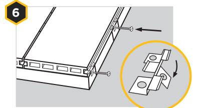
In order to fit the final board, bend the Slim Clip screw hole to a **90° angle** and fit over the edge of the subframe. Screw into place to secure boards. If necessary, you can trim the excess tabs off.
