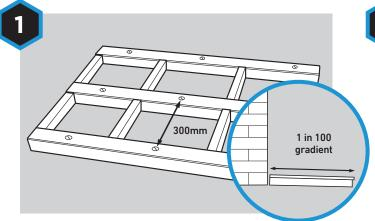
We recommend using a similarly fire rated subframe and allow for a gradual gradient of at least 1 in 100 (1%) that runs away from any adjoining buildings. Boards should run lengthways down this gradient to help water naturally disperse.
