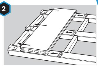
We recommend adding **HD Protect™** Premium Joist Tape to the top and exposed cut ends of the timber to protect it from moisture that can cause rot and loosening of screws.
