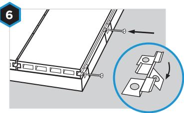
In order to fit the final board, bend the Slim Clip screw hole to a 90° angle and fit over the edge of the subframe. Screw into place to secure boards. If necessary, you can trim excess tabs off.
