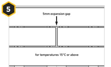
**IMPORTANT:** Do not allow deck boards to meet at the ends. When installing in temperatures of:
