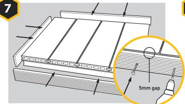
If using Fire Fascia, drill pilot holes with counterbore through the fascia at 200-300mm intervals. According to ambient temperature allow a **5-7mm gap** between end of deck board and the fascia. Screw fascia to the joist. Always screw fascia to the joist at a 90° degree angle.
