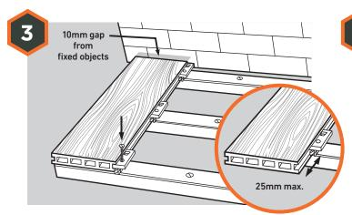
To secure the first board, use one Universal Clip and screw on every joist. Take a screw, place in the hole located in the Universal Clip and screw into the wooden joist. **Do not tighten at this stage**. Make sure the boards do not overhang the joist at the edge by more than 25mm and a 10mm expansion gap should be left between the
