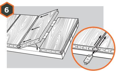
To fit the final boards, first measure the width of the final two boards to find out where the outer edge of the final board will lie. Using these marks, fit starter clips and slot the final board into place. Now insert the penultimate board, slide down the required number of Universal Clips and screw these into place.
