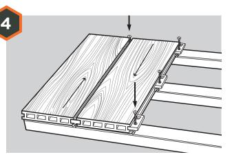
Take the next piece of deck and securely push into the Universal Clips. Now nip the screw to secure the Universal Clip against the board. **Do not over tighten**. Repeat steps 3 and 4 to cover the deck, using one Universal Clip and screw on every joist.
