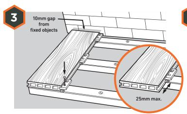
To secure the first board, use one Universal Clip and screw on every joist. Take a screw, place in the hole located in the Universal Clip and screw into the wooden joist. **Do not tighten at this stage**. Make sure the boards do not overhang the joist at the edge by more than 25mm and a 10mm expansion gap should be left between the wall or other fixed objects surrounding the deck.
