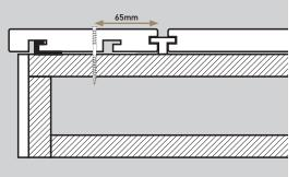
After installing the *HD Deck Dual*<sup>®</sup> bullnose deck board, as per the above instructions, use the Universal Clip to secure to the rest of the deck. See **Using the New Universal Clip** overleaf.
