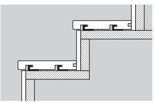
Install the *HD Deck Dual*<sup>®</sup> bullnose deck board as per the above instructions, leaving a gap behind the board to enable you to fit the fascia.
