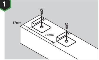
Place two starter clips as shown in the above diagram and secure in place with the respective screws. Ensure that the spacing measurements are correct.
