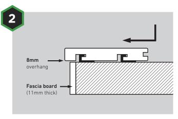
Insert the *HD Deck Dual*<sup>®</sup> bullnose deck board over the clips and push it forward. Secure in place with Universal Clips as required.
