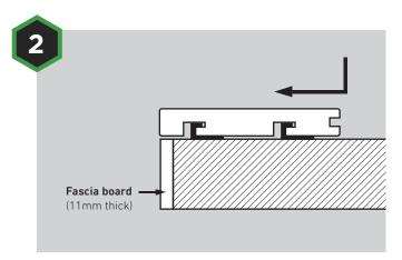
Insert the *HD Deck Dual*<sup>®</sup> bullnose deck board over the clips and push it forward. Secure in place with Universal Clips as required.
