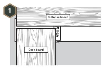
Insert the Universal Clip as shown in the diagram with the front of the clip positioned in the groove of the secured bullnose deck board.
