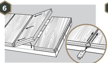
To fit the final boards, first measure the width of the final two boards to find out where the outer edge of the final board will lie. Using these marks, fit starter clips and slot the final board into place. Now insert the penultimate board, slide down the required number of Universal Clips and screw these into place.
