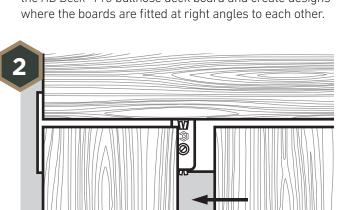
Screw the Universal Clip to the joist, then securely push the next deck board in place.
