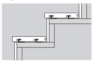
Install the *HD Deck® Pro* bullnose deck board as per the above instructions, leaving a gap behind the board to enable you to fit the fascia.
