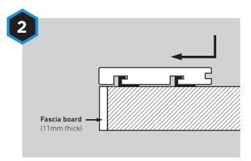
Insert the *HD Deck XS*<sup>®</sup> bullnose deck board over the clips and push it forward. Secure in place with Universal Clips as required.
