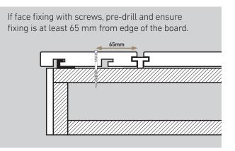
After installing the *HD Deck XS*<sup>®</sup> bullnose deck board, as per the above instructions, use the Universal Clip to secure to the rest of the deck. See **Using the New Universal Clip** overleaf.
