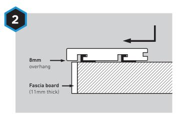
Insert the *HD Deck XS®* bullnose deck board over the clips and push it forward. Secure in place with Universal Clips as required.
