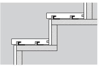
Install the HD Deck  $XS^{\otimes}$  bullnose deck board as per the above instructions, leaving a gap behind the board to enable you to fit the fascia.
