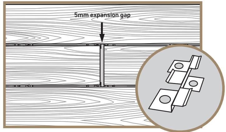
**SLIM CLIP ALTERNATIVE:** The Slim Clip can be used to close up the gaps between boards if preferred. Simply follow Steps 1-5, using the Slim Clip in place of the Universal Clip. **IMPORTANT:** the expansion gaps at the ends where the deck boards meet, must be maintained as explained in Step 5, .
