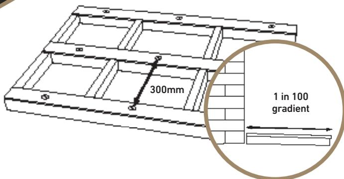
We recommend using treated 47x100mm timber joists and building in a gradual gradient of at least **1 in 100** (1%) that runs away from any adjoining buildings. Boards should run lengthways down this gradient to help water naturally disperse.
