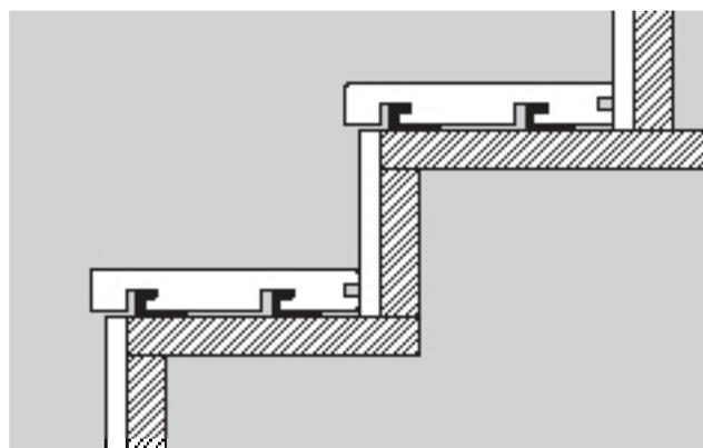
Install the *HD Deck® Pro* bullnose deck board as per the above instructions, leaving a gap behind the board to enable you to fit the fascia.
