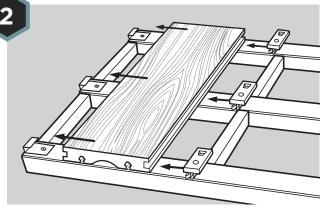
Place the first piece of decking on the timber frame with the decking running perpendicular to the joists. The first piece of deck may be secured with starter clips. **Do not** screw or nail through HD Deck® Clik, use one Universal Clip and screw on every joist.
