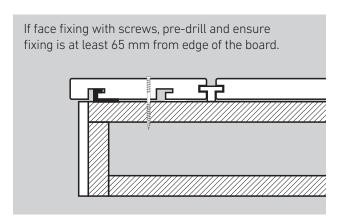
After installing the *HD Deck 150*® bullnose deck board, as per the above instructions, use the Universal Clip to secure to the rest of the deck. See *Using the New Universal Clip* overleaf.
