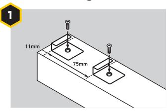
Place two starter clips as shown above, and secure in place with the respective screws. Ensure that the spacing measurements are correct.
