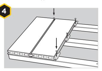
Take the next piece of deck and securely push into the Universal Clips. Now nip the screw to secure the Universal Clip against the board. **Do not over tighten**. Now repeat steps 3 and 4 to cover the deck, using one Universal Clip and screw on every joist.
