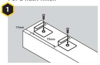
Place two starter clips as shown in the above diagram and secure in place with the respective screws. Ensure that the spacing measurements are correct.
