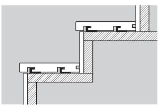
Install the HD Deck  $150^{\circ}$  bullnose deck board as per the above instructions, leaving a gap behind the board to enable you to fit the fascia.
