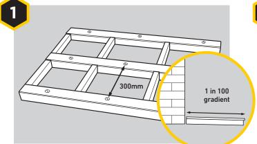
We recommend using treated 47x100mm timber joists and building in a gradual gradient of at least **1 in 100** (1%) that runs away from any adjoining buildings. Boards should run lengthways down this gradient to help water naturally disperse.
